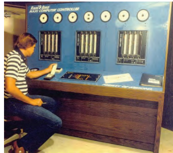
First Central Control System. "Maxi" - 1978
