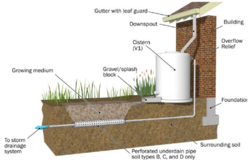
Figure 1-6. Cistern with Bioretention BMP Example Illustration
